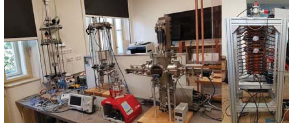
Fig. 1. From left: Paschen curve, resonance cavity, probes stand. Right panel: linear magnetic trap.
