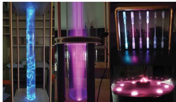
Fig. 2. From left: iodine tube, tube with variable pressure and one electrode; from top: set of spectral tubes, resonance cavity with plasma.
