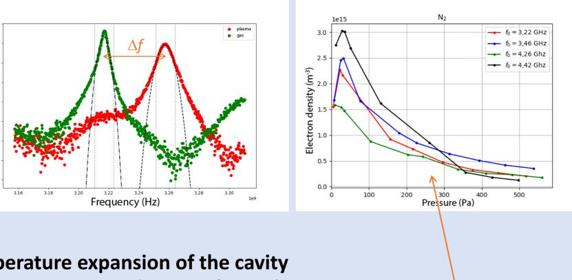
• Plasma was generated 11 times for 30 s by power 70 W • After that, the frequency was measured for another 15 minutes
